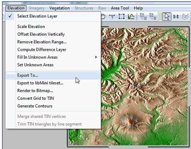
Elevation data are saved in ArcInfo-ASCII-format by selection of menu *“Elevation / Export to ...”*
