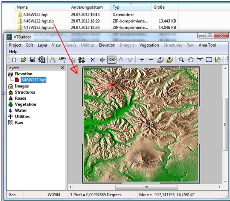
After start of VTBuilder you have to load the hgt-file. The easiest way is to pull and drag the unpacked (!) hgt-file (here N46W122.hgt.zip) into the window of VTBuilder.
