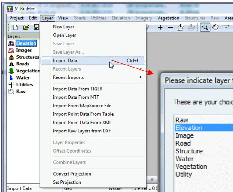
As a second way to load the elevation data file select menu "**Layer / Import Data**". In the following window select layer type "**Elevation**". After <Ok> you select the unpacked hgt-file for import, not the packed zip-file. This seems to work with Vista too.
