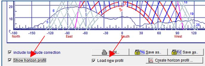
6. Now you can switch on/off the horizon profile with mouseclick on checkbox "*Show horizon profile*" (left red arrow above).
